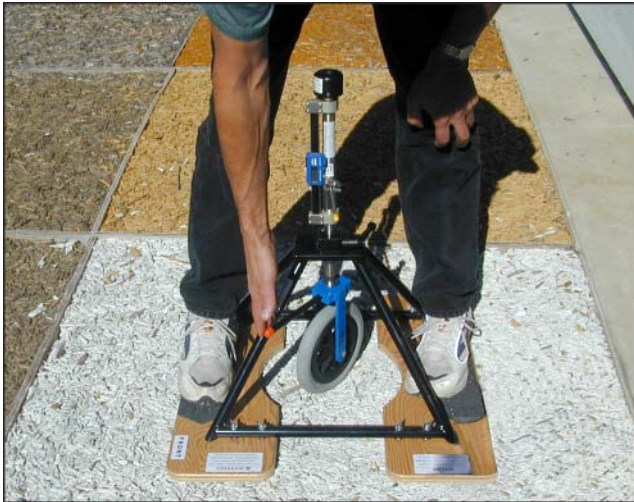
Figure 3—Rotational penetrometer in use on surface A2.
