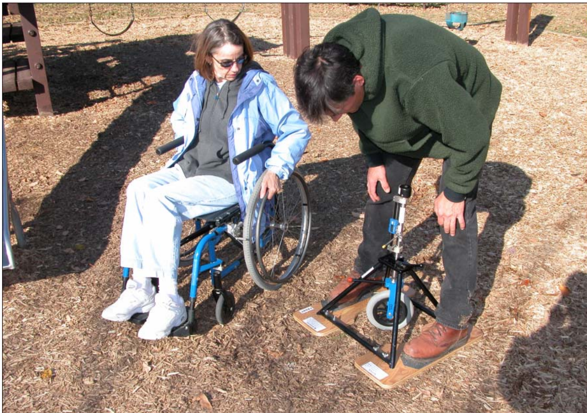
Figure 9—Measurement of accessibility with rotational penetrometer.
