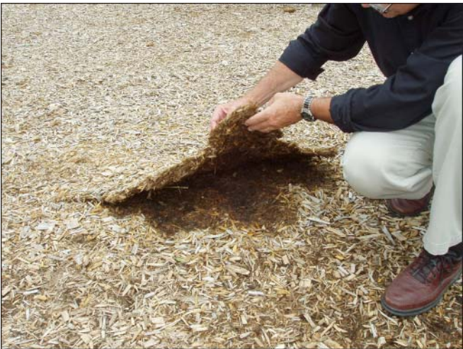
Figure 14—Exposed and torn edge of Vitri-Turf SEWF.
