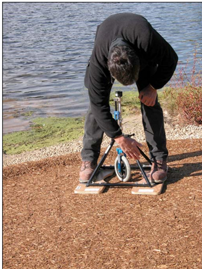
Figure 14—Rotational penetrometer used to measure accessibility.
