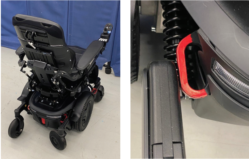
FIGURE 2-5 Power wheelchair with four securement points (red) required by WC19 for a four-point WTORS.
