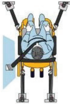
FIGURE 2-4 Four-point, strap-type wheelchair tiedown and three-point belt occupant restraint system.
