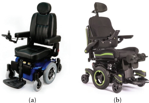
FIGURE 2-1 Examples of (a) a basic power wheelchair, which generally has no seat functions and may be used by people who can sometimes stand and walk short distances; and (b) a power wheelchair equipped with powered seating functions for people with significant disabilities.
