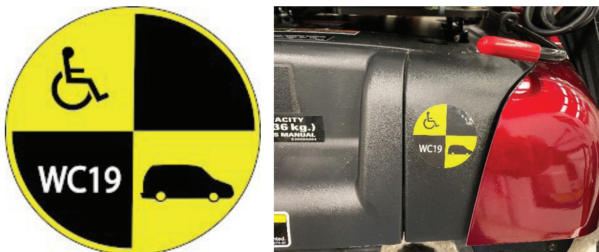
FIGURE 3-4 RESNA WC19-compliant label and its application on a power wheelchair.
