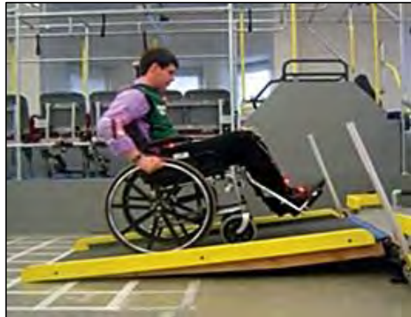
A study participant tests a ramp with a 1:8 slope using a manual wheelchair.
